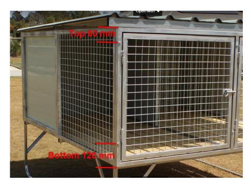
**Step 2.** Ensuring you assemble the unit upside down, the bottom of the frames should be facing up, with the large hole distance at the top. Ensuring the left and right panels have the green side of the colorbond sheet facing outwards (screws to the inside) attach the MESH END of the 2 side panels to the gate assembly using M10 x 75mm bolts. Fingertighten only.
