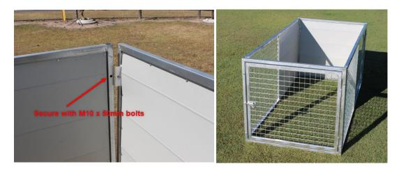
**Step 4.**Measure the diagonal corners of the unit, adjusting until the measurements are the same and the frames are square. Then tighten all bolts firmly.
