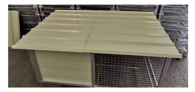
When roof sheets are correctly in place, screw the sheets to the bearers and rear frame with the self-tapping screws provided. Note - there are enough long roof screws to screw through each ridge section across the middle only (on the overlap of front and rear sheets). The shorter screws are designed to be used in the gullies front, middle and back. Be mindful not to screw through the roof sheets into the access holes in the top of the bearers.
