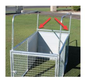
Place the other ends of the skids into the frame and secure the front floor brace in the same manner (on the INSIDE of the skids), then push both ends of the 2 skids full into the frames and ensure the floor braces are seated firmly on the frames. Attach the middle floor brace with the 75mm bolts. There are 2 sets of holes that the middle floor brace can bolt to – you can bolt this to either the front or back set of holes. Finger-tighten only.
