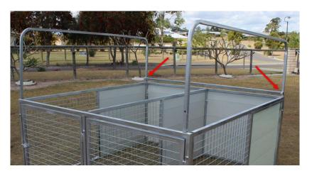
Place the other ends of the skids into the frame and secure the front floor brace to the **INSIDE** of the skids in the same manner. There are 2 sets of holes that the middle floor brace can bolt to – you can bolt this to either the front or back set of holes, noting the middle floor brace bolts into the middle panel as well. Finger-tighten only.
