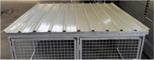
When roof sheets are correctly in place, screw the sheets to the bearers and rear frame with the self-tapping screws provided. Note - there are enough long roof screws to screw through each ridge section across the middle only (on the overlap of front and rear sheets). The shorter screws are designed to be used in the gullies front middle and back. Be mindful not to screw through the roof sheets into the access holes in the top of the bearers.
