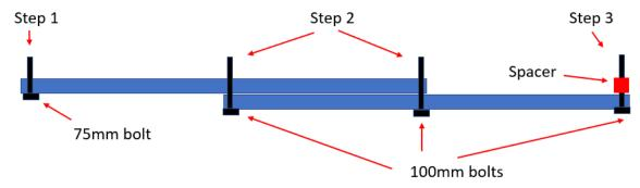
Referencing the diagram and pictures above, align the left side rear floor brace first, using a 75mm bolt to attach the left side to the skid. Then place the right side brace in front of the left brace and line the holes up. Using 100mm bolts, bolt the right floor brace through the left brace and then through the skids in the 2 middle sections only. Then use a 100mm bolt and 30 x 30mm spacer to secure the right hand side floor brace to the skid as per picture above. Finger-tighten bolts only.
