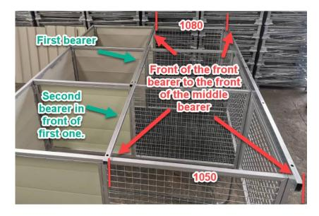
The second middle roof bearer Must go in FRONT (towards the front of the kennel, see pic above) of the first middle roof bearer that was measured back 1080mm (this second bearer will be 1050 from the front of the front bearer). Then use the self-tapping screws to secure the L brackets to the bearers and outer frames.
