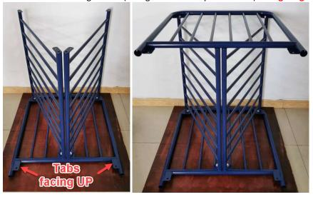
**Step 3.** Insert the feed tray with the shiny side facing UP and screws underneath when standing upright. Secure with M10 x 25mm bolts and ensure the bolt threads are facing INWARDS. This is designed to be a snug fit - if need be, loosen off the bolts on the 2 hay racks to allow the feed tray to slide into position, then tighten all bolts firmly.
